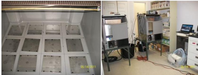
Figure 1: Coupon and lab set-up of ice machines.
